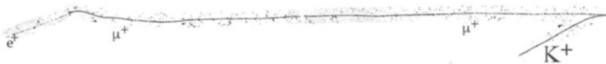
Fig. 2.12 Decay K^+ \rightarrow \mu^+ \nu of a stopping kaon in a nuclear emulsion. A mass of 562 \pm 70 MeV was estimated from multiple scattering and the energy loss derived from the grain density (adapted from [21])
